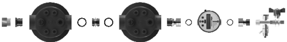
Obr. 2: Montáž armatury → také obr. 1 Fig. 2: Assembling the fitting → also Fig. 1
